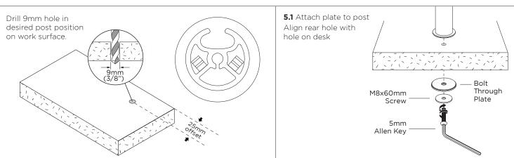
5. Installing bolt through
